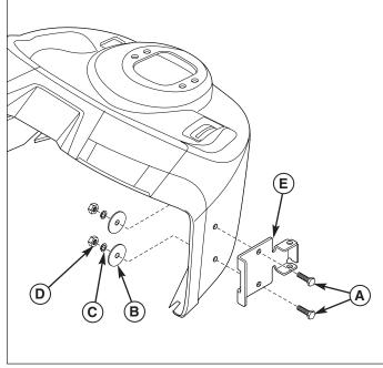
Figure 29. Mount Control Bracket - Current Models A. 1/4-20 x 7/8 Capscrews
